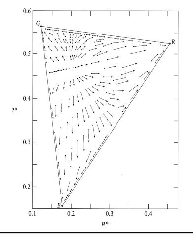
Shifts in reproduced chromaticities resulting from uncompensated gamma of 1.273 (such a gamma is desirable to compensate the contrast lowering in the dim surround).
