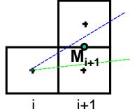
IF  $(d_{i+1} \le 0)$  // Increment in x only i  $d_{i+2} = d_{i+1} + a = d_{i+1} + dy$  // Incremental calculation ELSE // Increment in x and y  $d_{i+2} = d_{i+1} + a + b = d_{i+1} + dy - dx$  y = y + 1ENDIF x = x + 1
