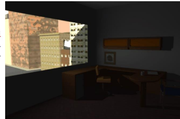
A linear mapping of the luminances that underexposes the view of the interior.
