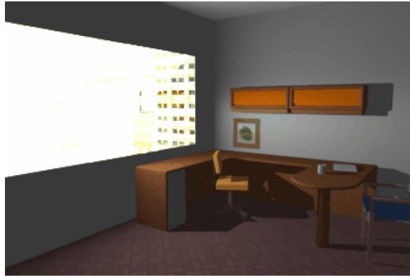
A linear mapping of the luminances that overexposes the view through the window.
