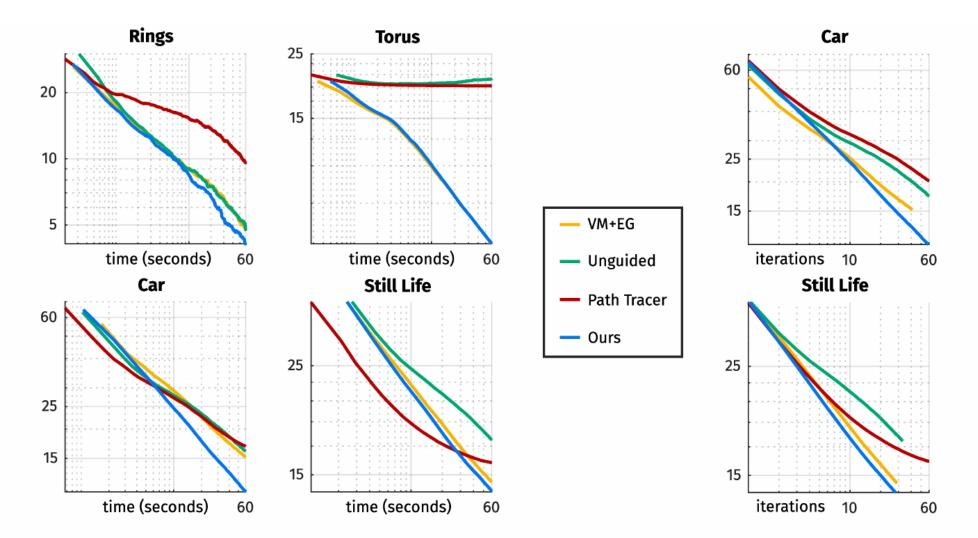
**Figure 11:** *Equal-time (one minute) and equal-iteration-count convergence rate (log-RMSE) for some of our test scenes. Our method has either better or identical convergence rates in all our test scenes, even on a per-iteration level.*
