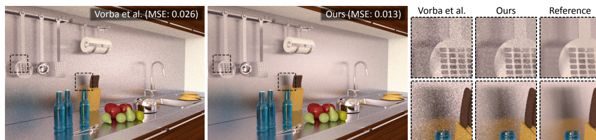
Figure 8: In scenes with glossy surfaces, product importance sampling (HEV + 16) (right) yields higher sample quality (512 samples) over pure radiance based path guiding (VKŠ + 14) (left).
